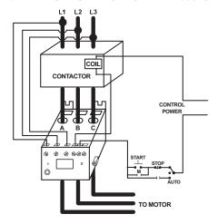
CURRENT TRANSFORMER WIRING DIAGRAM OR MODEL 777-ACCUPOWER
