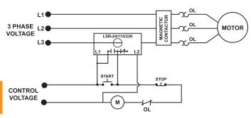
TYPICAL WIRING DIAGRAM FOR OVERLOAD DETECTION
