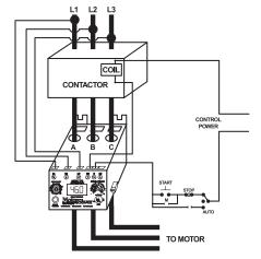
CURRENT TRANSFORMER WIRING DIAGRAM FOR MODEL 777 (80 to 800 amps)
